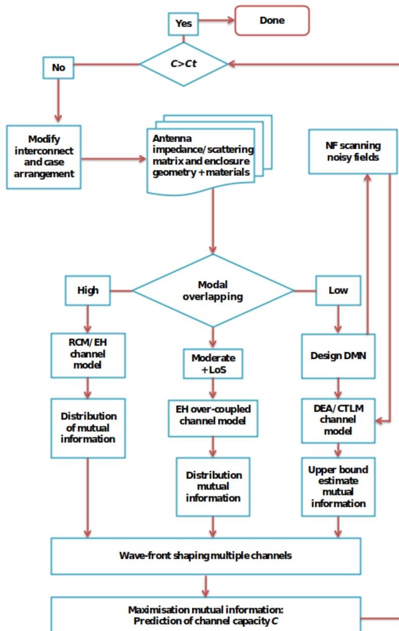
Figure 5 Workflow chart for far-field C2C communications link in enclosures
