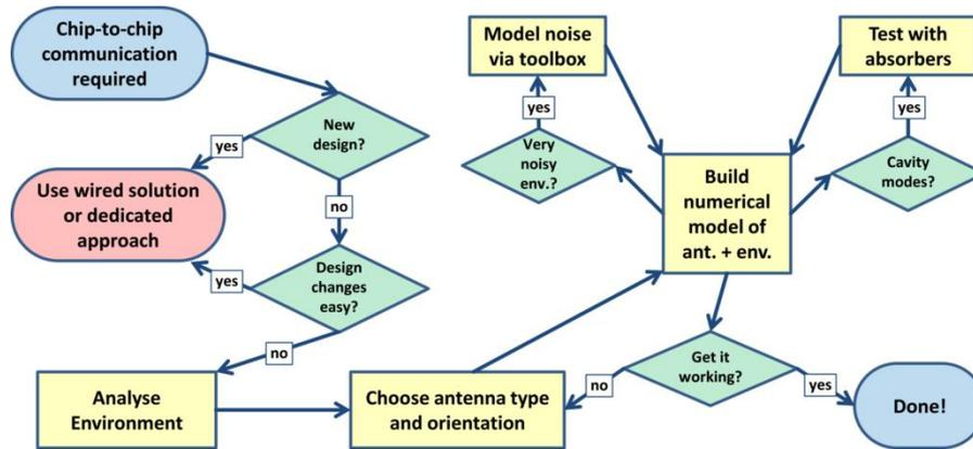
Figure 2 Proposed workflow for designing a wireless C2C communications link in the General Scenario
