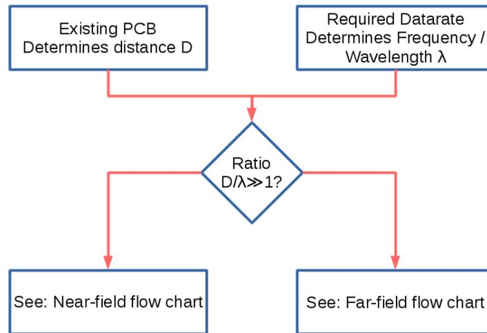
Figure 3 Proposed workflow for designing a wireless C2C communications link for the DS
