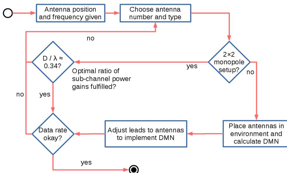
Figure 4 Proposed workflow for designing a near-field DMN
